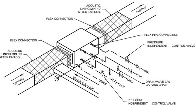
**FAN COIL (4 PIPE), WITH GRISWOLDS DETAIL**
