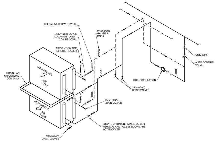
**AIR HANDLER COIL PIPING DETAIL**
